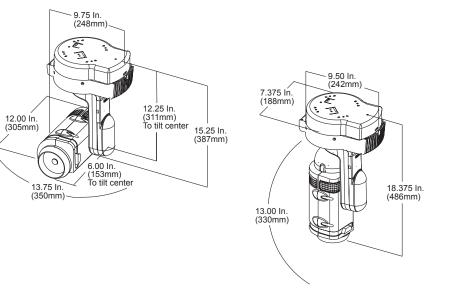
**Note:** AR50s must be installed with the base in a horizontal position. Failure to do so will shorten fixture life and violate warranty
