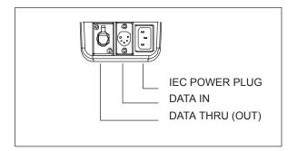
A 100 ohm 1/4 watt termination resistor must be mounted in a 5-pin male XLR connector and inserted into the DATA THRU connector at the last luminaire in each data run to terminate DATA (+) and (DATA (-) lines together.
